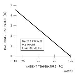
FIGURE 5. Maximum Power Dissipation vs T<sub>AMB</sub> for the TO-263 Package
