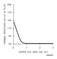
FIGURE 6.  $\theta_{\text{(J-A)}}$  vs Copper (2 ounce) Area for the SOT-223 Package
