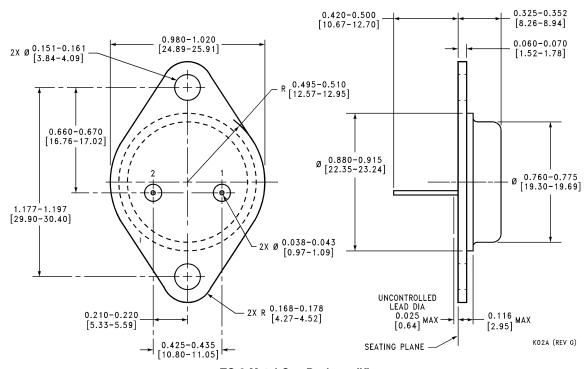
TO-3 Metal Can Package (K) Order Number LM117K STEEL, LM117K STEEL/883, or LM317K STEEL NS Package Number K02A
